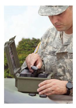
RadLight Reader is engineered to withstand extreme environmental conditions experienced by firefighters and emergency responders LANDAUER's dosimetry devices employ patented optically stimulated luminesence (OSL) technology, provding the highest accuracy of total accumulated dose possible. RadLight Reader is designed to work with the RadWatch Dosimeter and operates with OSL technology.
