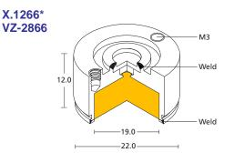
\* X.1266 manufactured according to drawing VZ-2866
